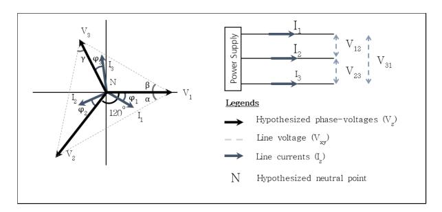
B2.3 The total power factor can be obtained by the equation B1. The active power (P) can be read from the metering devices based on two-wattmeter method.
